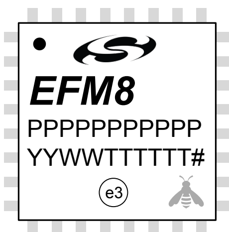
Correct QFP32 Package Marking
